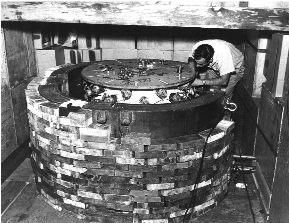
Fig. 15 - Reines and Cowan's neutrino detector
