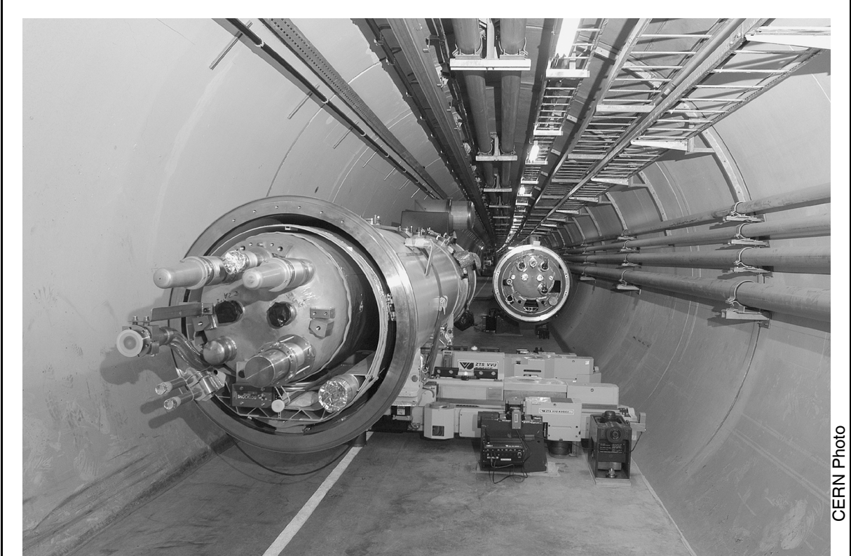
Fig. 62 - The LHC tunnel with a superconducting magnet
