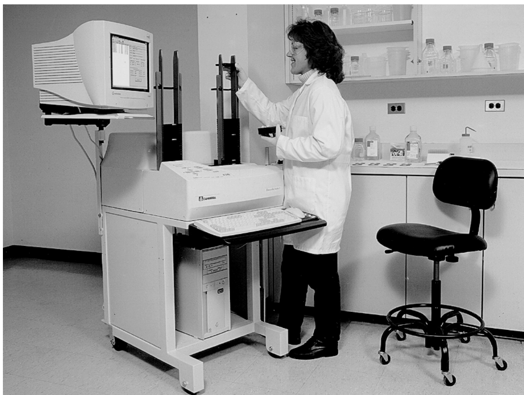
Fig. 22 - A commercial alpha/beta wipe counter
