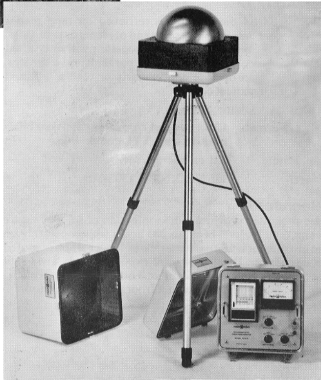
Fig. 14 - A commercial pressurized ion chamber instrument
