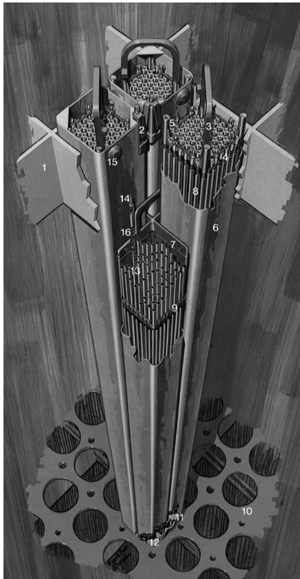
Fig. 14 - A BWR fuel assembly
