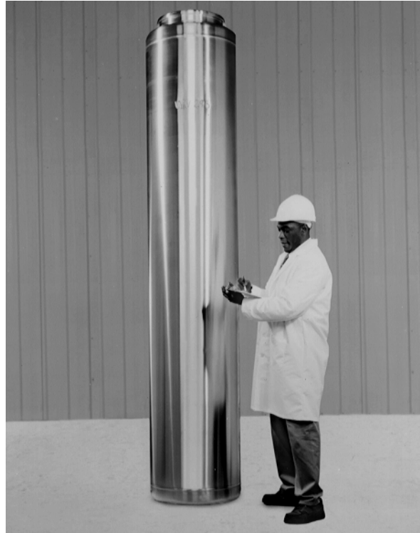
Fig. 8 - West Valley canister for vitrified high level radwaste
