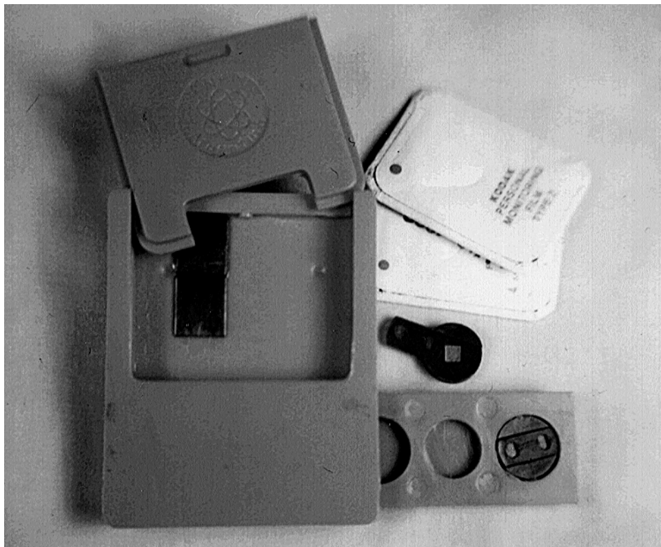
Fig. 45 - A hybrid badge using film and TLD
