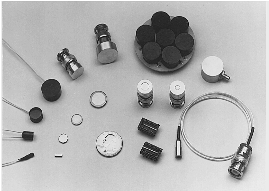
Fig. 60 - Examples of CZT radiation detectors
