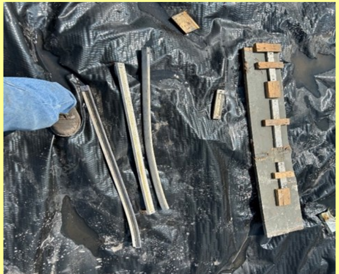
Radium Static Eliminators, Dose Rate: ~800 mrem/hr @ 30 cm
