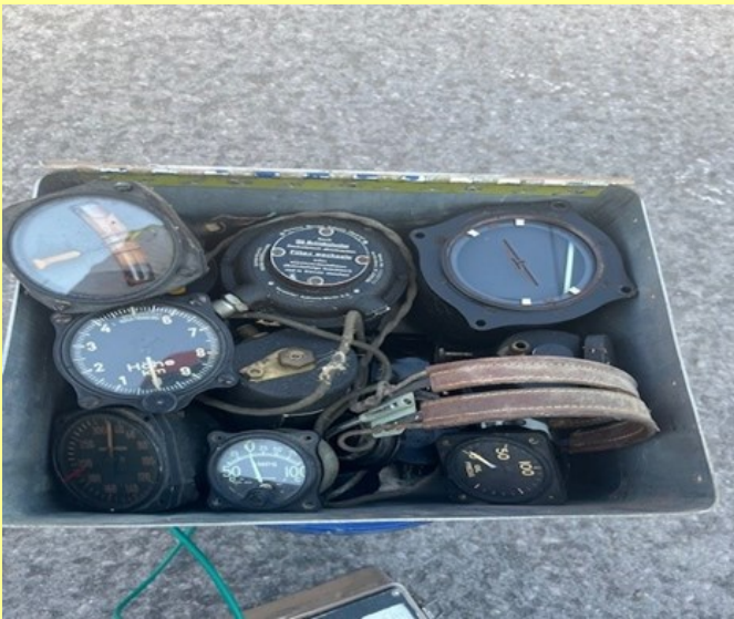
Radium Military Gauges , Dose Rate: ~150 \mu rem/hr on contact
